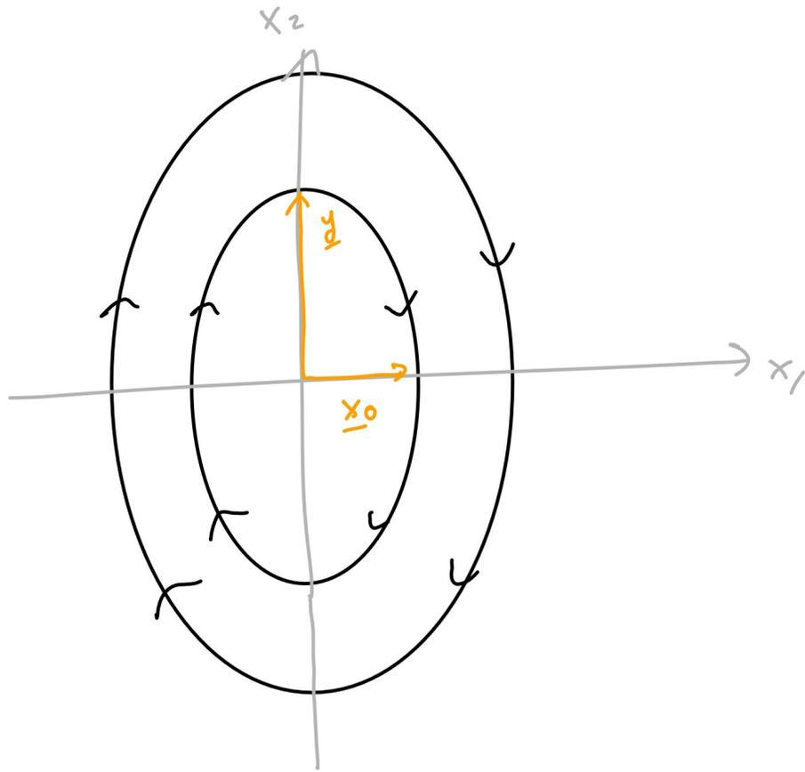
Flow lines are ovals. Keeping track of only the  $x_1$ -coordinate, we see sinusoidal oscillation:
