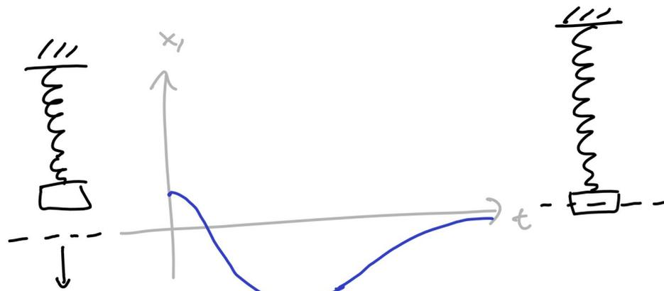
This kind of flow line corresponds to the other characteristic motion of an overdamped harmonic oscillator (passing through its rest point once).
