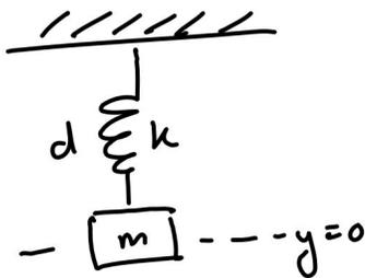
$$\omega_0 = \sqrt{\frac{k}{m}}, \quad \gamma = \frac{d}{2m}.$$
