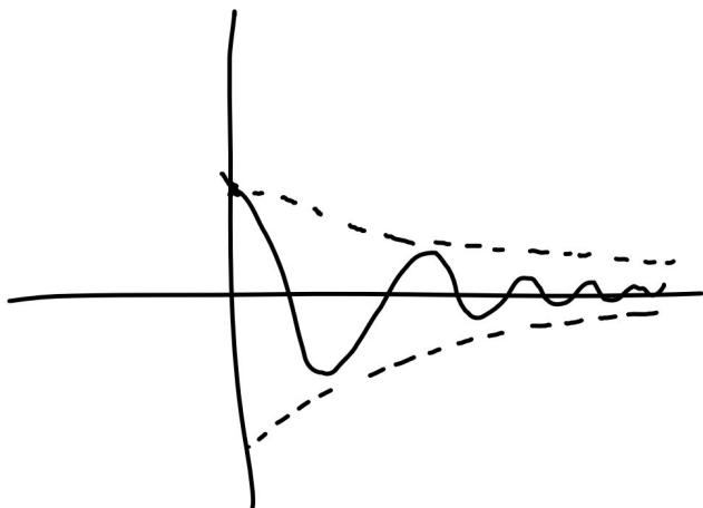
The spring-mass system is said to be underdamped
