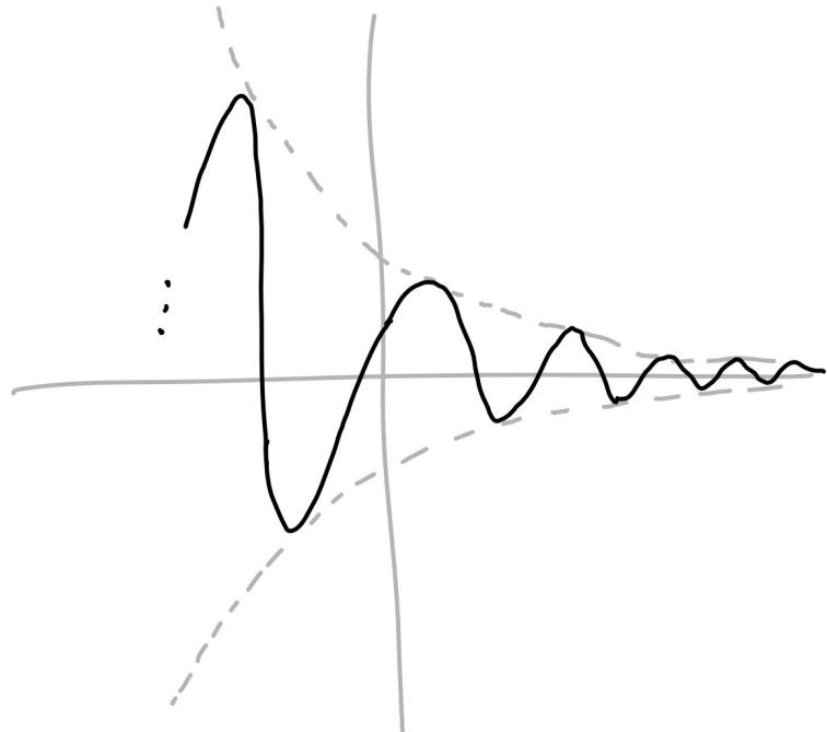
Let's interpret these solutions in terms of the behaviour of a damped spring-mass system (an example of a damped harmonic oscillator)
