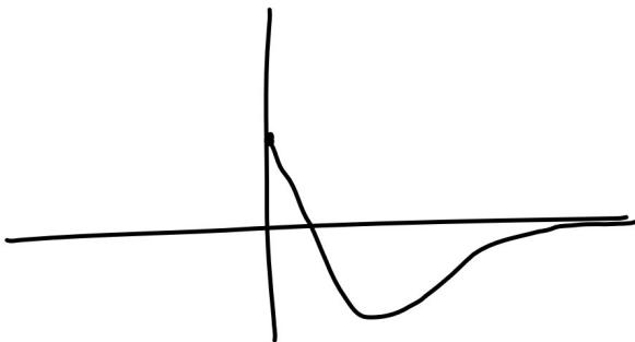
The spring-mass system is said to be critically damped in this case.
