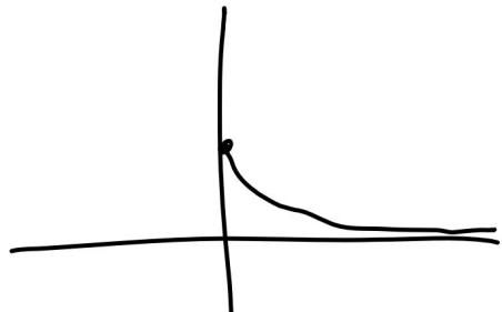
In this case, the spring-mass system is said to be overdamped.
