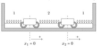
Suppose that each spring has the spring constant given by the number above that spring in the diagram. Suppose that the mass of each block is equal to 1. Neglect friction.
